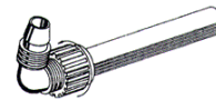
Step 3 Slide the nut to the threads and tighten securely to the fitting
